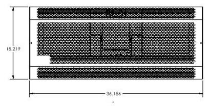
Mount to wall or ceiling using QTY 4 5/16" bolts or threaded rod. MOUNT 2" INWARD OF DOOR OPENING
