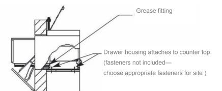
RA-LGTD18X14X9 is shipped pre-assembled and ready to install.
