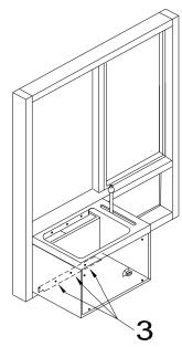
REMOVE THE 3 SCREWS HOLDING THE DRAWER ASSEMBLY TO THE WINDOW SUPPORT ANGLE.
