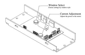
The Window Select Dial is used to set the type of door configuration for the model of window.
