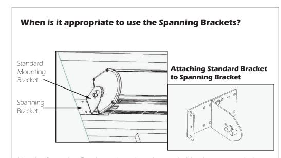
Use the Spanning Brackets when there is no suitable place to attach the Standard Brackets above or behind the unit. Or stated another way, when the only suitable attachment surface is out to the side of the unit.
