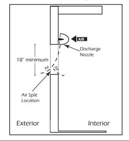
Rotate the Air Curtain by adjusting its position in the mounting brackets so the split location is at the base of the window.
